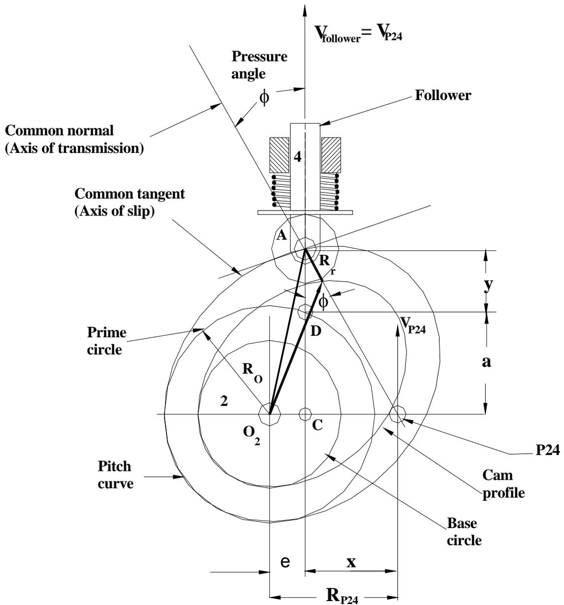
**Figure 1:** Plate Cam in Contact with Reciprocating Roller Follower
