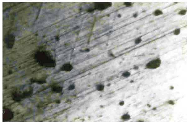
Figure 13: Homogenized @8000 (1hr) Etched in Acidified Iron(111) Chloride. (X100).
