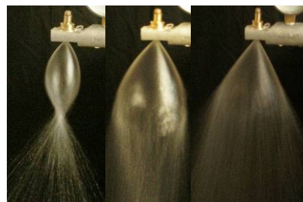
Figure 5: Spray Formation Stages Regarding to Fluid Swirl.
