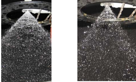
Figure 6 and 7: Spray Angle of Internal (Left Photo) and External Nozzle (Right Photo).
