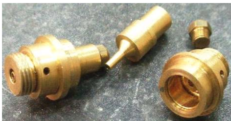
Figure 2: Assembled and Disassembled of a Manufactured Swirl Injector.
