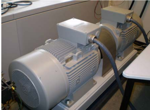
Figure 1: Photograph of the 37kW Induction Motor for Wind Turbine Emulator (WTE), Directly Coupled to a Generator.
