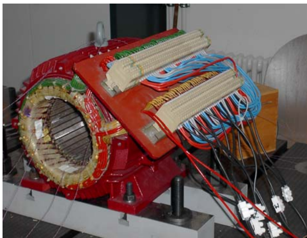
Figure 8: Stator part of the test machine showing the installed J-type thermoelements.
