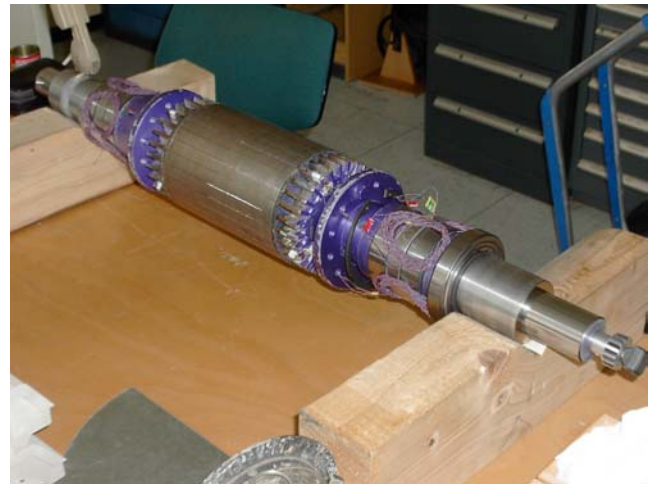
Figure 9: Rotor part of the test machine showing the installed J-type thermoelements.
