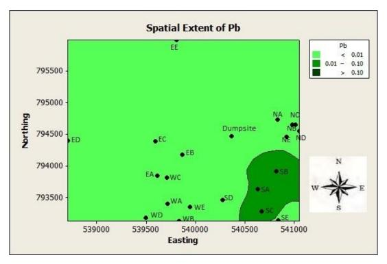
Figure 7: Spatial Variations of Lead (Pb) in Groundwater around the Dumpsite.
